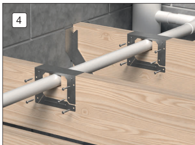
Bend the relief tab inwards against the joist and fasten the bracket into the face of the joist using the screws included in the kit
