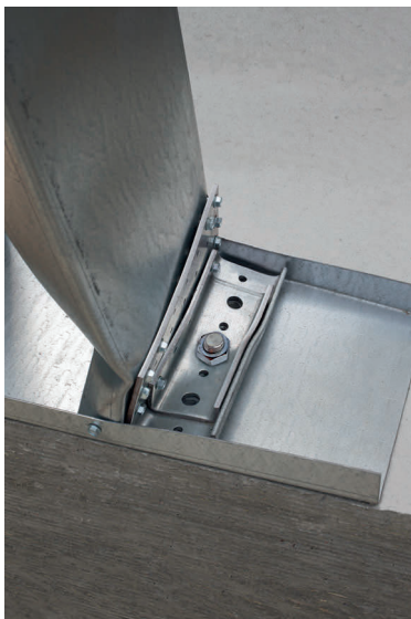
Assembly test with member failure
